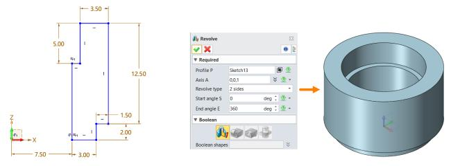
Figure 190 Sketching the Revolve Profile
