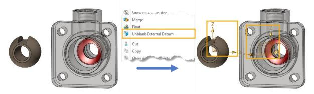
Figure 260 Unblank external datum
