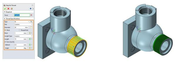
Figure 146 Setting Thread Parameters
